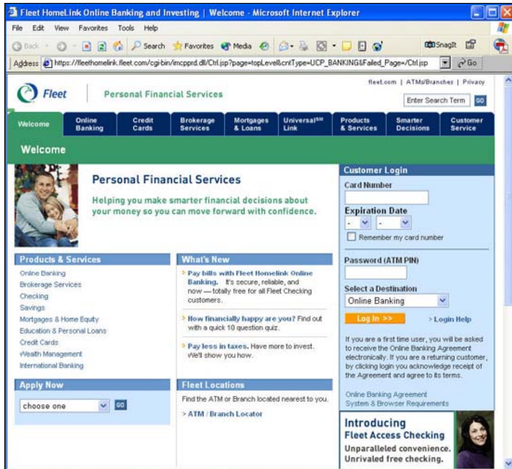
Figure 2: Fake Address Bar displayed. Notice the change in colour on the right? You can also observe if you click on the drop down arrow on the address bar, the history is empty.
